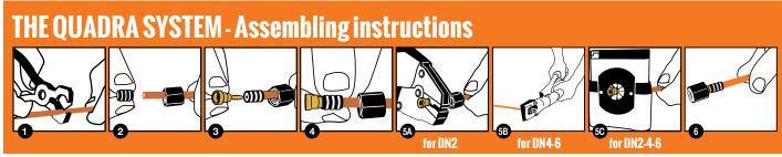
Cut the QUADRA capillary hose to the required lenght using the special WXAOO4 cutter Slip the nut over the hose (depending on fi tting type). Ensure that the threaded side is pointing towards the end of the hose that needs assembling.
